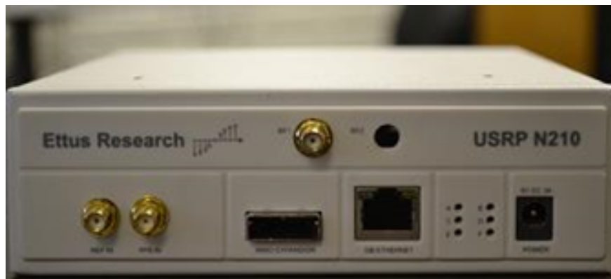
Figure 4.2: The USRP N210 from Ettus Inc. is used as the front-end to convert RF down to IF and save the IF samples to a hard drive.
